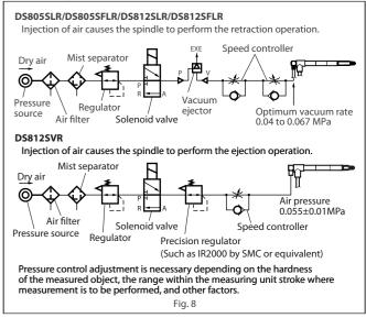
If the spindle ejection speed is too fast, an error may appear on the display the moment that the workpiece is touched. Excessive impact may dislodge the retainer inside the bearing, causing the measuring range to be reduced. In this case, use a speed controller as shown in Fig. 8 to adjust the spindle speed.
