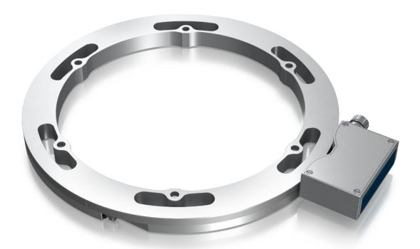
Some motors require a speed feedback sensor mounted on the main shaft between other parts in the machinery. Here the shaft dimensions may be large — sometimes around a meter — which means that a standard optical encoder is not suitable. Therefore Leine & Linde has developed a new series of bearingless encoder rings, the 2000 series. It has several features specially designed to meet the demands found in heavy industries.
