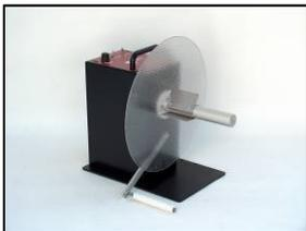
**UCAT-2:** This powered Unwinder automatically tracks label usage and provides powered label feed at speeds up to 76cm /sec (30-ips). The **UCAT-2** accepts standard 76mm (3”) cores and rolls up to 300 mm (12”) in diameter. 255 mm (10”) width is available. It can also be used as a full-featured Label Rewinder without any special setup. LABELMATE's renowned Constant Adjustable Torque™ control system allows precise adjustment of feed speeds and rewind torque. External STOP / RUN Input included.
