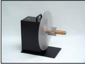
**UCAT-S:** This is the world's least expensive professional Unwinder. It is unpowered and has a trouble-free fixed brake. The UCAT-S accepts up to 300 mm (12”) diameter rolls and up to 155 mm (6”) width, 76mm (3”) cores.
