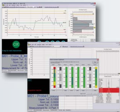
Software tools for data capture and data analysis (settings, measurements, inspection reports). See chapter A – Connectivity
