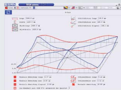
Measurement of a granite plate according to U-Jack
