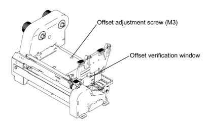
The relationship between the offset adjustment screw and the print head heating element is shown below:
