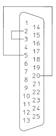
Fig. Loopback test
